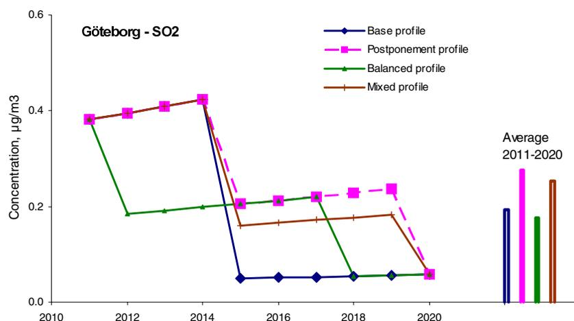
**Figure 3.4.** Concentration of SO<sub>2</sub> which can be attributed to ship emissions for Göteborg. The vertical bars indicate the average concentration over the period 2011-2020.
